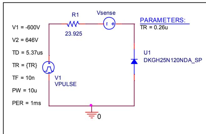
Test condition:  $V_{CC} = -600, 646$  (V),  $I_C = 25$  (A),  $-di/dt = 200$  (A/us)
