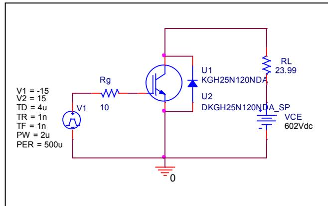
Test condition:  $I_C=25$  (A),  $V_{CC}=600$  (V),  $V_{GE}= \pm 15$  (V),  $R_G=10$  ( $\Omega$ )
