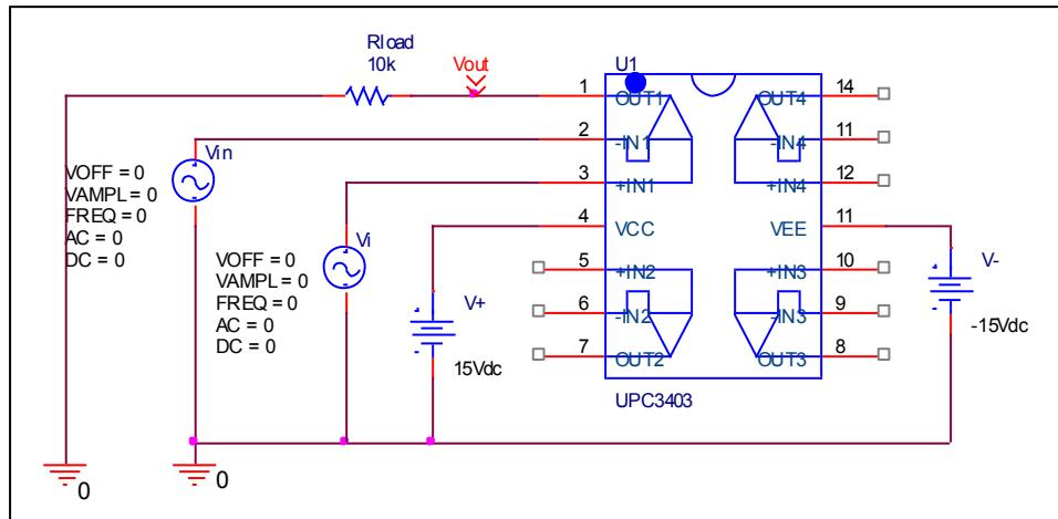
The output voltage change of Opamp(open loop) when input DC voltage ( $V_{in} - V_i$ ) is changed with the evaluation circuit is simulated
