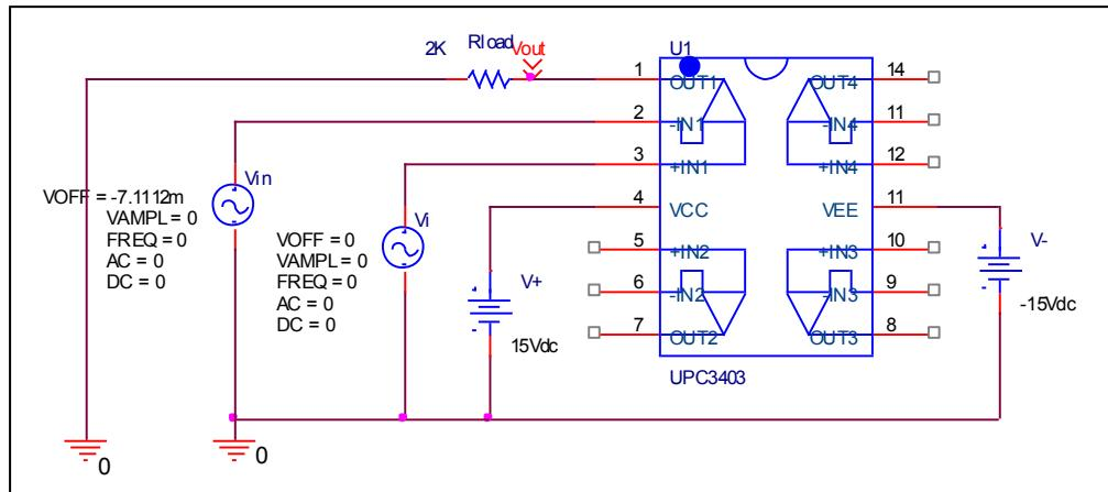
The input offset current when supply voltage to op-amp
