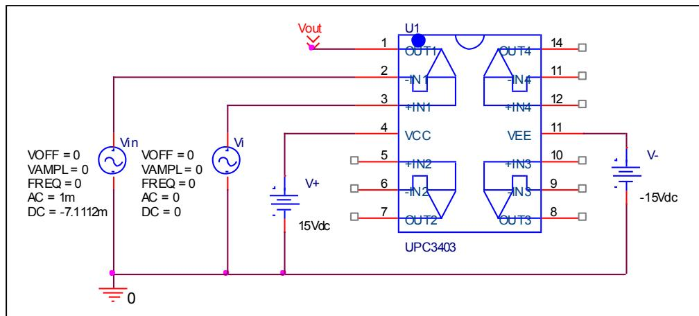
The open loop voltage gain of op-amp when supply AC input voltage 1MHz frequency
