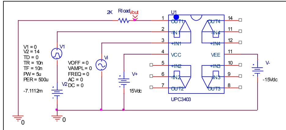
The output voltage change versus time (slope) of op-amp when input electric step voltage.
