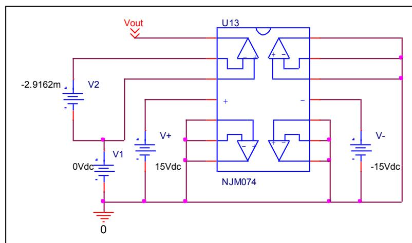
Common Mode Reject Ratio =  $272113.444 / 52.35 = 5197.964 = 74.316\text{dB}$
