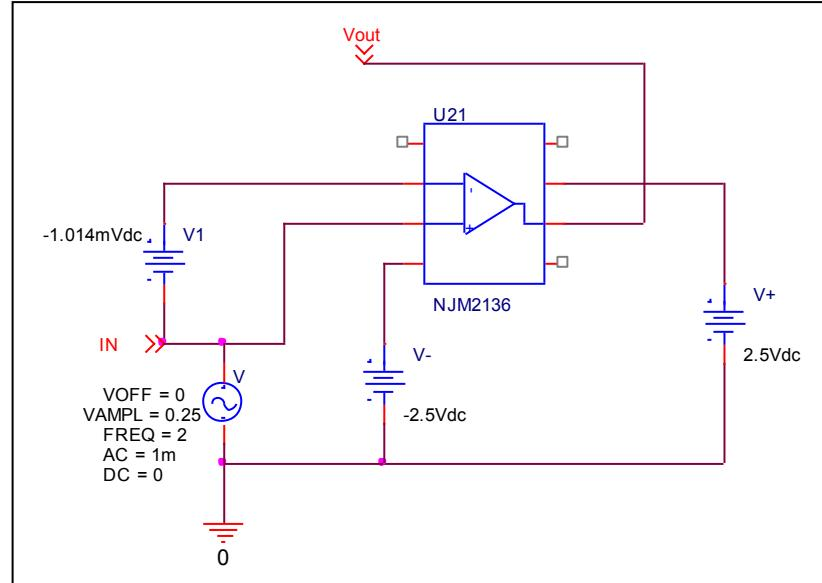
$$\text{Common Mode Reject Ratio} = 5043.7 / (2.485 / 0.5) = 1014.83$$
