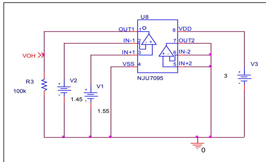
$$V_{IN+} = (V_{DD}/2) + 0.05, \quad V_{IN-} = (V_{DD}/2) - 0.05$$
