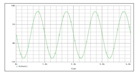
Common mode gain=12.462/0.4 =31.155 Common Mode Reject Ratio=199215/31.155=6394.31 Change to dB = 20log(6394.31) = 76.1 dB
