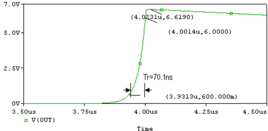
**V<sub>o</sub>=6.619(V)** at V<sub>i</sub>=20(V), C<sub>t</sub>=0.2u(F)
